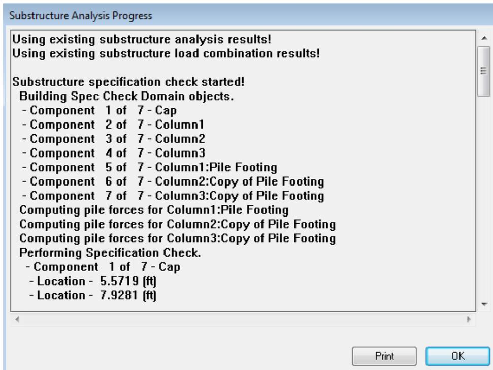
The engineer can use this process to fine-tune the design. After you find reinforcement and dimensions that satisfy the specification articles, you can do a final finite element analysis and spec check.
