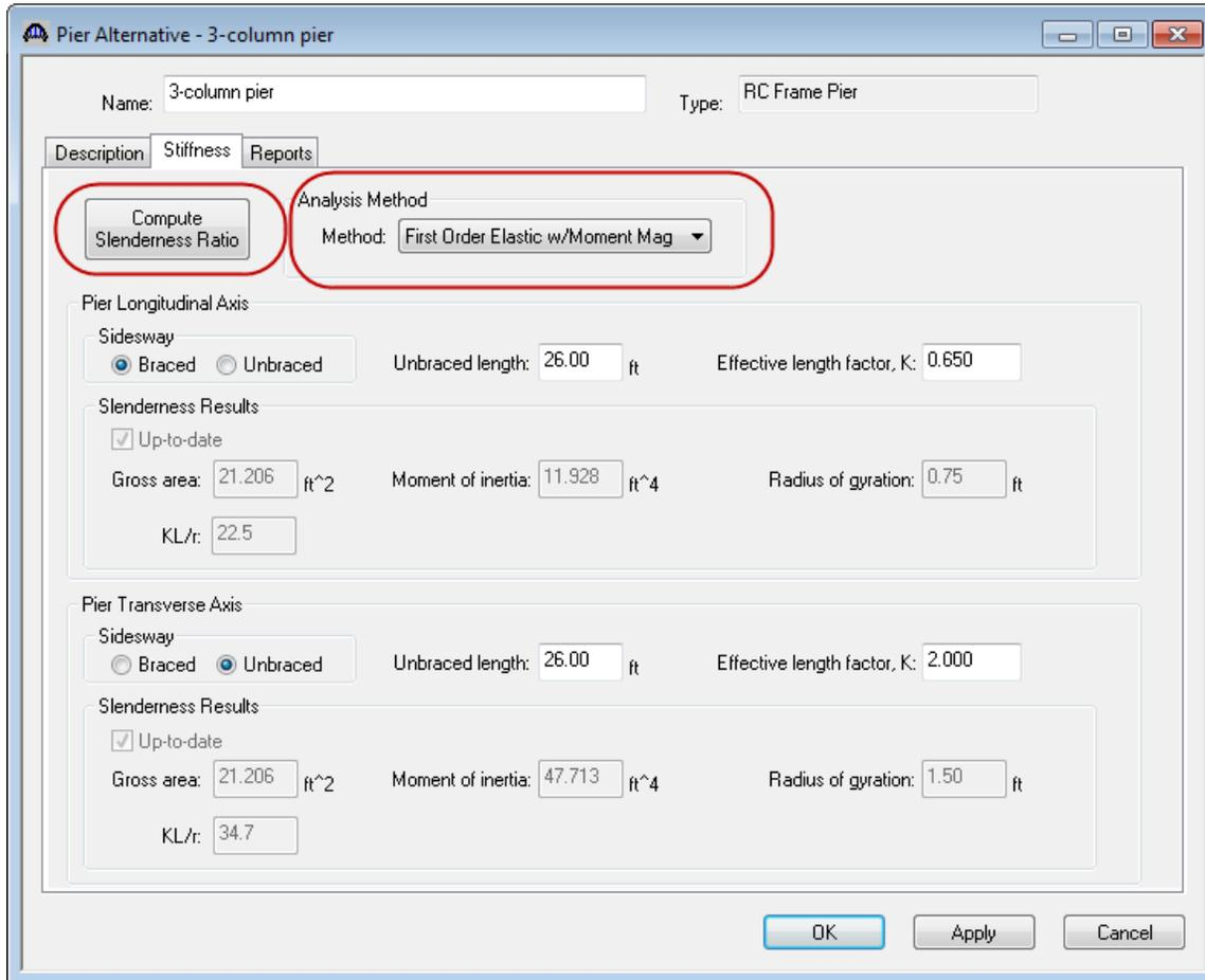
In this example, we should consider moment magnification to account for the effects of slenderness. Launch a spec check of the pier from the Substructure toolbar.
