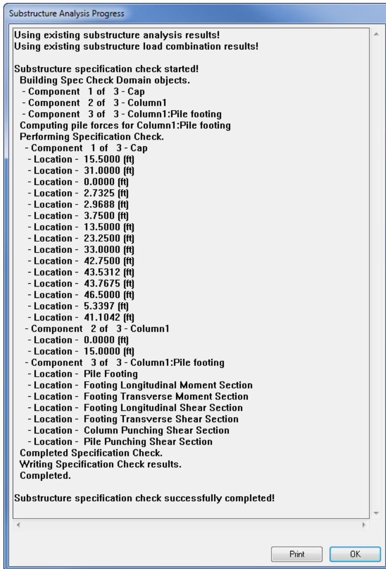
Fig4. Substructure Analysis Progress Window
