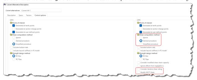
These options are applicable when **General procedure** - Shear computation method is used. Select these options to perform iterative shear rating and consider modifying the MCFT theta value and view results as discussed in previous sections of this tutorial.
