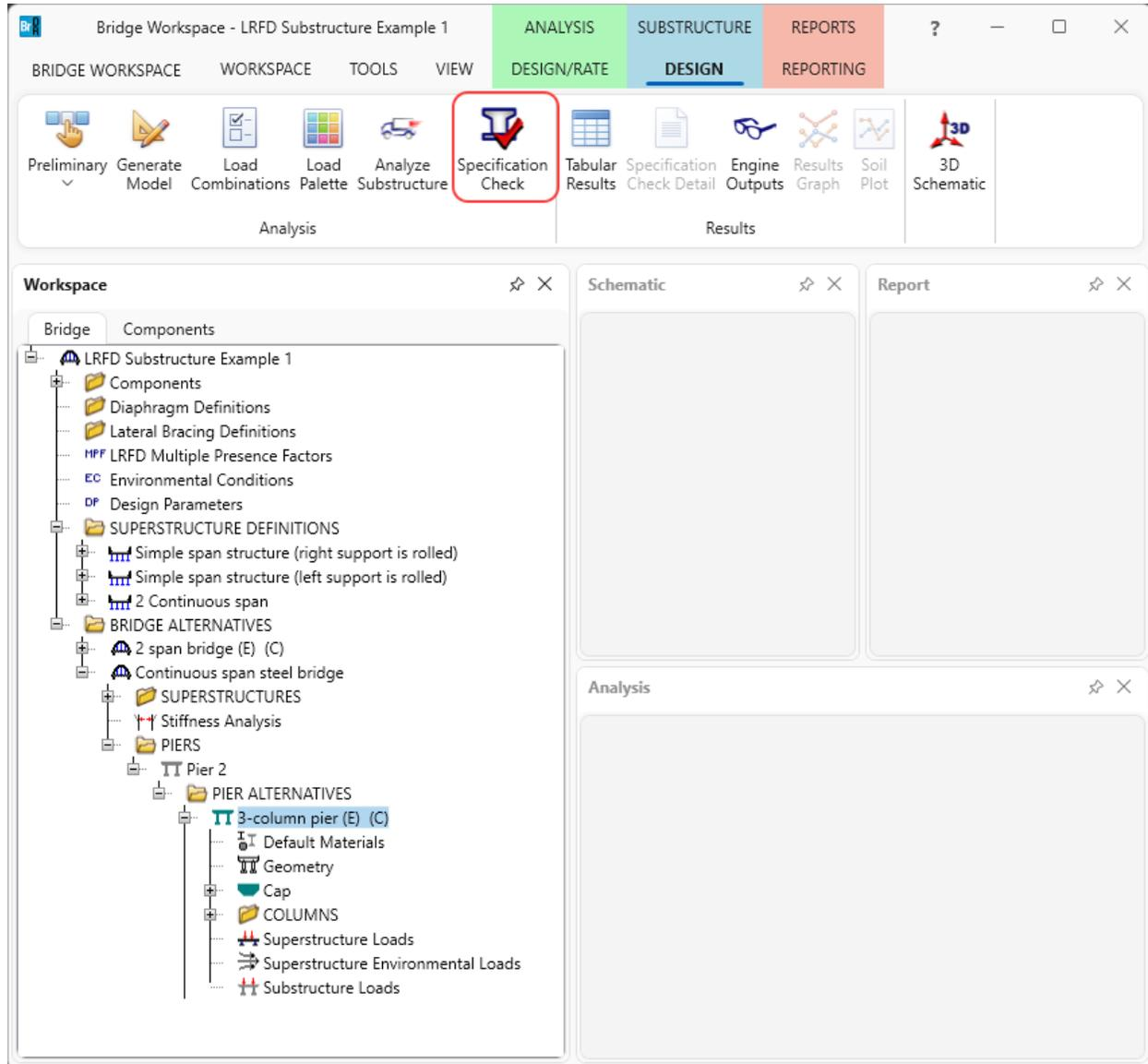
The superstructure will first be analyzed to determine the superstructure dead load reactions. The remaining loads acting on the pier (such as live load, wind, etc.) are computed and applied to the pier finite element analysis. Load combinations are generated and then the specification checks are processed.
