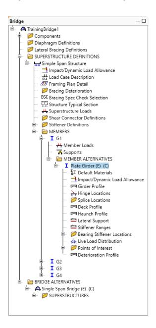
Select member alternative Plate Girder (E) (C). From the Analysis group of the DESIGN/RATE tab on the Bridge Workspace ribbon, click on the Analysis Settings button to open the Analysis Settings window.
