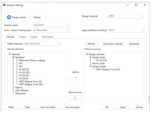
Navigate to the **Output** tab as shown below. Select **Fatigue stress ranges** report and **Service II stresses ranges** report by checking in check box under **AASHTO engines reports**. Click the **OK** button to save and close the **Analysis Settings** window.
