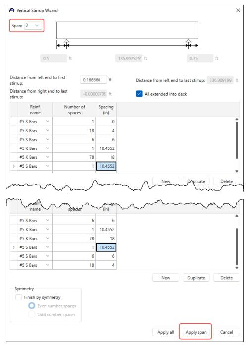
Click **Apply all** and the wizard closes returning to the **PS Shear Reinforcement Ranges** window populated as shown below.
