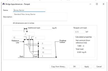
The parapet properties are copied to the Bridge Appurtenances - Parapet window as shown below.
