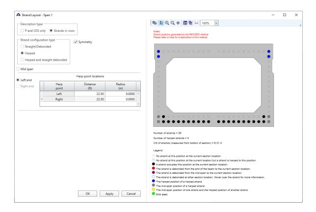
Enter the following data for Spans 2 and 3 in the same manner as described above. **Span 2** is shown below, **Span 3** has the same information as Span 2.
