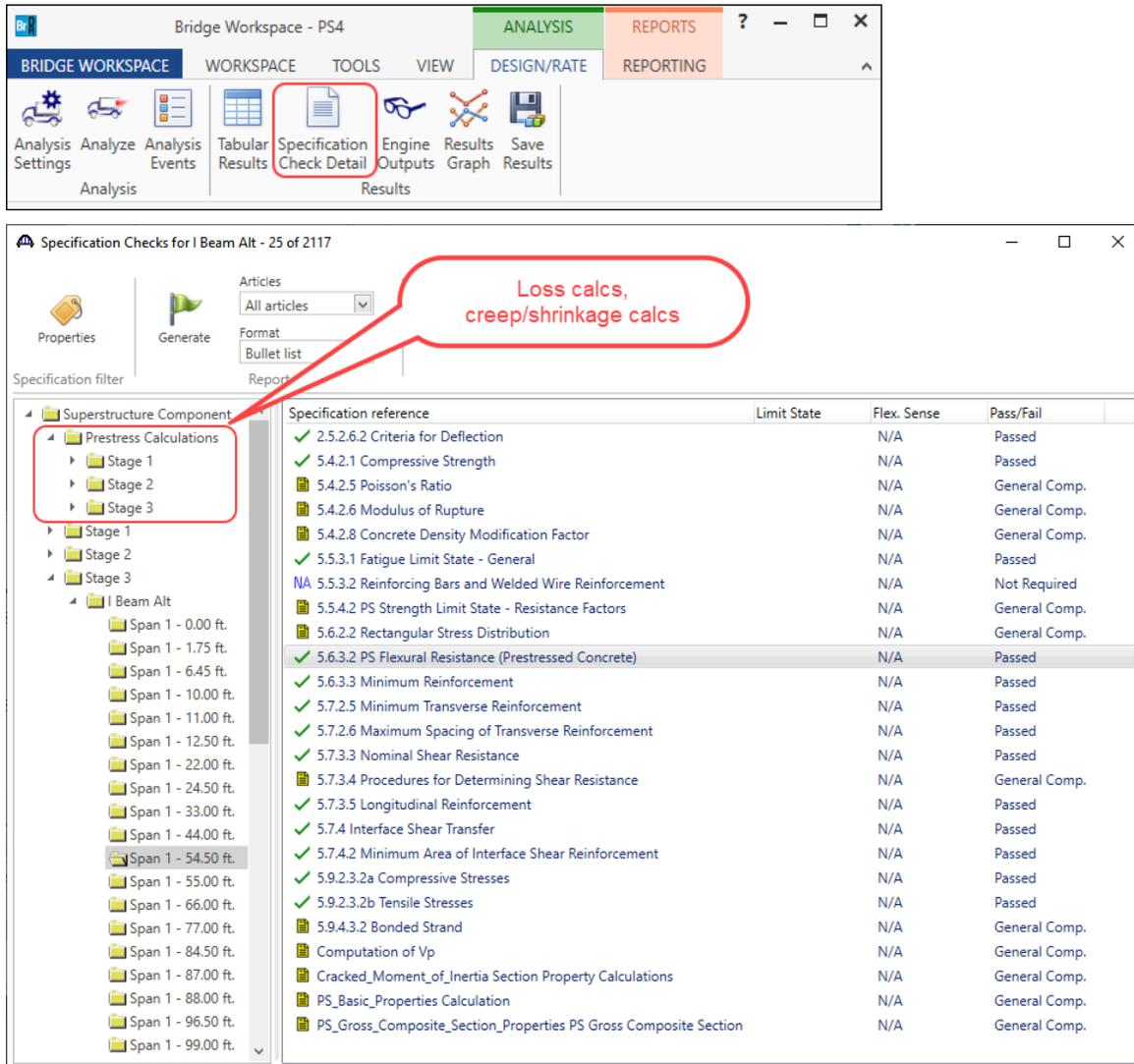
Open the spec check detail window for the flexural resistance at the middle of simple span 1. The following is noted for this window, other spec articles are similar:
