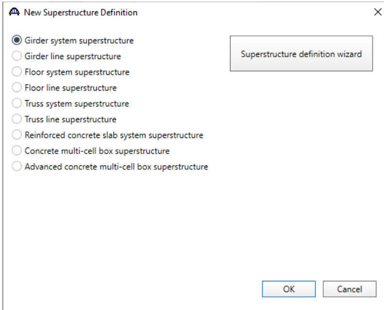
Select **Girder system superstructure**, click **OK** and the **Girder System Superstructure Definition** window will open.
