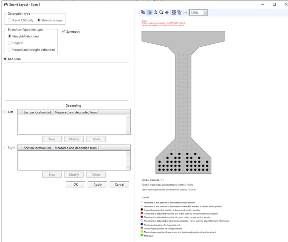
Now select the **Left end** radio button Under the Debonding section, select **New** to enter a left debonded section location as **273 inches**. This distance is measured from the left end of the precast beam. The strands can be defined at the left end of the span by selecting strand locations in the right hand schematic. Define the following debonded strands at this location.
