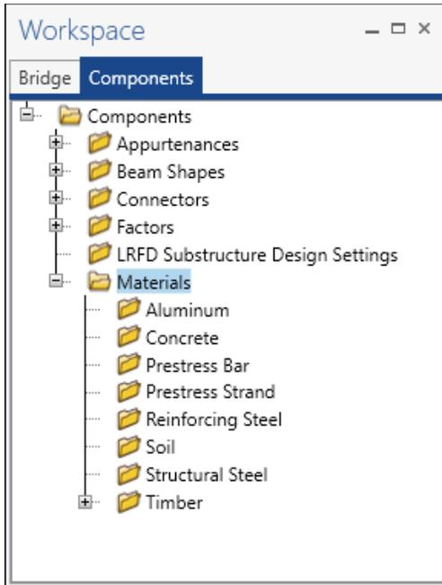
To add a new concrete material, in the **Components** tab of the **Bridge Workspace**, click on **Materials**, **Concrete**, and select **New** from the **Manage** group of the **WORKSPACE** ribbon (or right mouse click on **Concrete** and select **New**). The window shown below will open.
