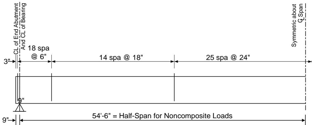
**Beam Elevation Showing Stirrups**
