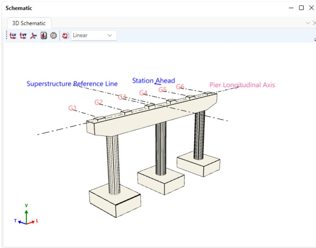
This tutorial discusses modeling the foundation for Column 1 as a drilled shaft instead of a spread footing.
