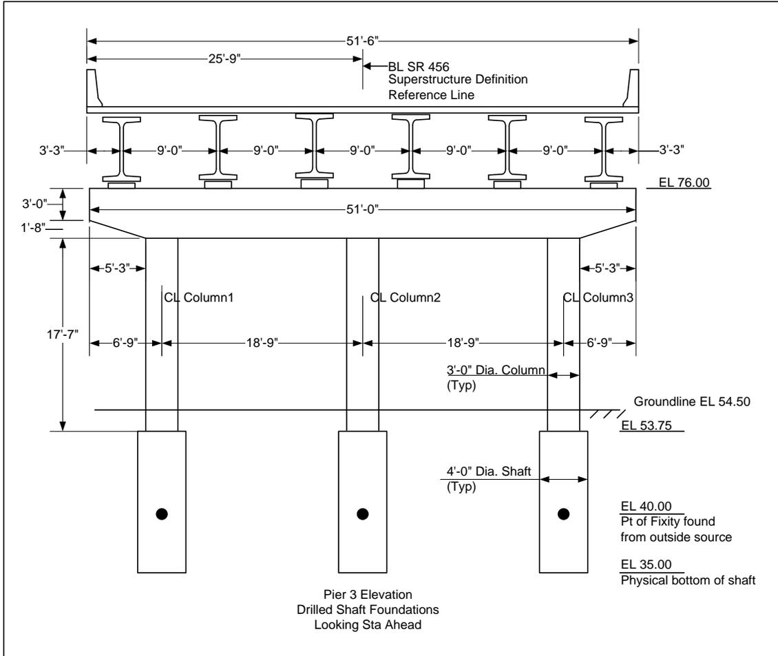
Pier Drilled Shaft Example
