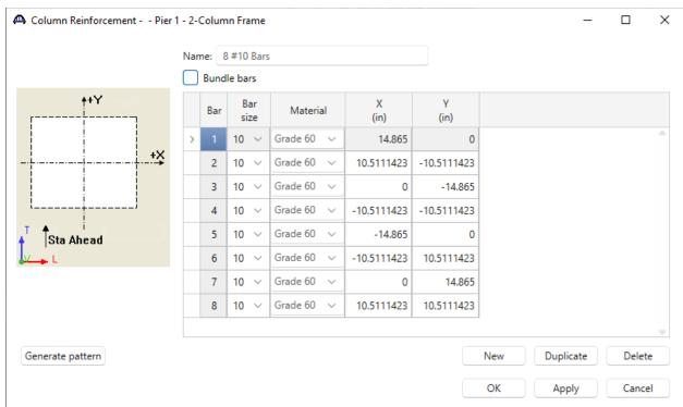
The following bar locations are generated for this pattern. Uncheck the **Bundle Bars** checkbox.
