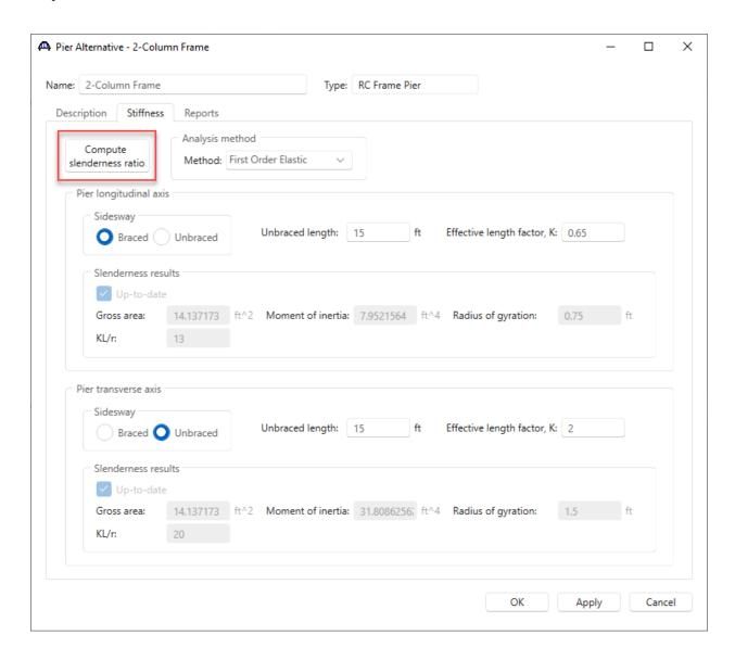
BrDR computes the KL/r ratios for the pier longitudinal and transverse axes based on the pier alternative geometry that was input. Independent evaluation of KL/r ratios can be done in accordance with AASHTO LRFD Article 5.7.4.3 to determine if the first order elastic analysis performed by BrDR is satisfactory for this pier.
