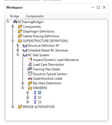
No changes are required in this window. The first **Member Alternative** created will automatically be assigned as the **Existing** and **Current** member alternative for this **Member**.
