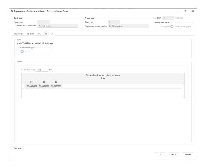
BrDR does not compute the superstructure shrinkage load. Values for these loads must be entered manually.
