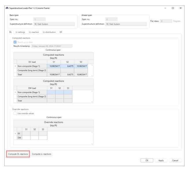
The **Override Reactions** grid permits to enter user-defined override values for the dead loads. Remember, these values will only be used in the pier finite element analysis if the **Use override values** box is checked on this window.
