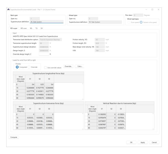
The top of the screen displays values computed by BrDR that are used to compute the wind on superstructure loads on the pier and in some cases lets the user override some of this data. The bottom of the screen displays loads on the superstructure members for wind blowing from left to right. The user can specify which direction the wind should blow in the actual pier finite element analysis in **the Load Combination Settings** window which will be discussed later in this tutorial.
