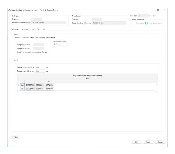
BrDR does not compute the superstructure temperature load. Values for these loads must be entered manually.
