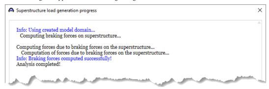
BrDR computes some of the superstructure loads on the pier for the user when the Superstructure Loads window is opened. This window lists details about how BrDR computes the loads and may contain warning and error messages. This window always appears after BrDR computes any loads for the user. Click **OK** to close this window.
