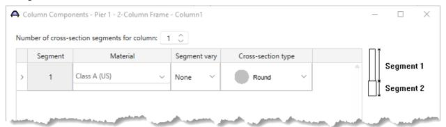
BrDR assumes the column cross section type is round when creating a new column. Since in this example the pier has round columns, this assumption is correct. Click the **OK** button to apply the data and close the window.
