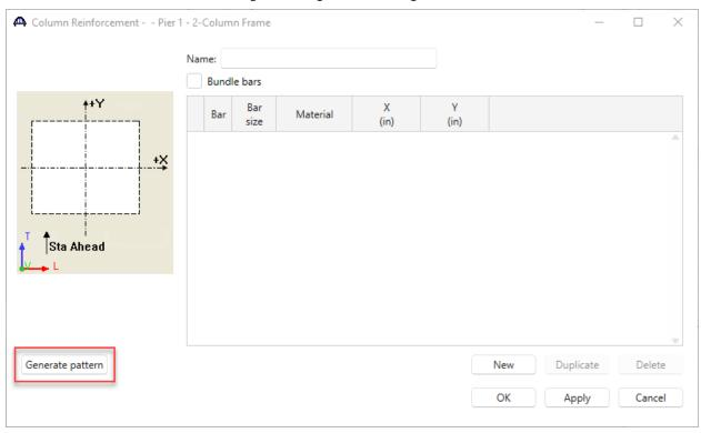
Click the **Generate Pattern** button above to use the pattern wizard to create a pattern of reinforcement. Enter the following data. The clear cover measured to the face of the flexural reinforcement is 2" cover to face of spiral plus ½" for the spiral diameter. After data is entered click the **OK** button.
