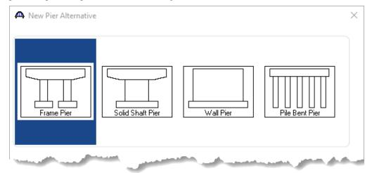
In this example, the two span continuous reinforced concrete slab system superstructure is supported by a 2-column frame pier. Select the **Frame Pier** and click the **Next** button.
