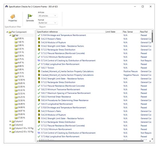
Double click on the article 5.7.3.2 Flexural Resistance (Reinforced Concrete) for Cap at location 0.00 ft
