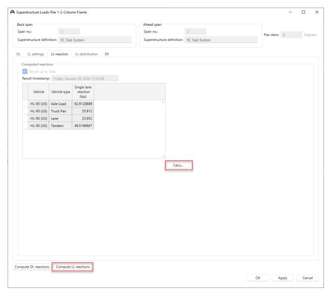
The vehicles used in the analysis are dependent on both the Design Mode selected on the **BrDR Substructure** ribbon and the **LRFD Substructure Design Settings** chosen on the **Pier Alternative: Description window**.
