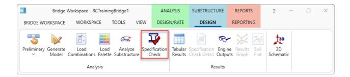
The **Validation** window will appear to alert the user to any missing data. Click the **Continue spec check** button to continue with the specification check.
