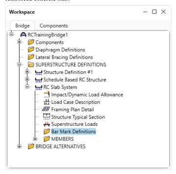
The bar mark definitions are used to describe a schedule of flexural reinforcement in the **Strip Profile** - **Reinforcement** tab. Input the data as shown below.
