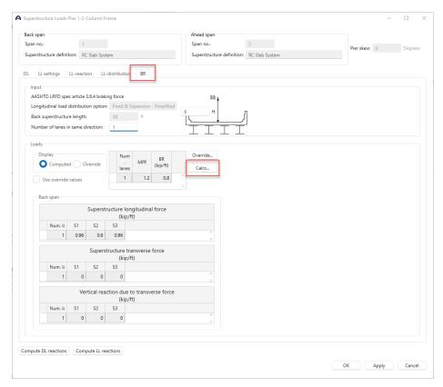
The Calcs button will open a report detailing the calculations BrDR performed to compute the friction forces.
