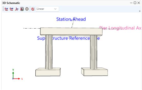
This 3D schematic is a to-scale drawing of the pier alternative. This schematic view has a lot of useful features like rotating, scaling, and dimensioning.
