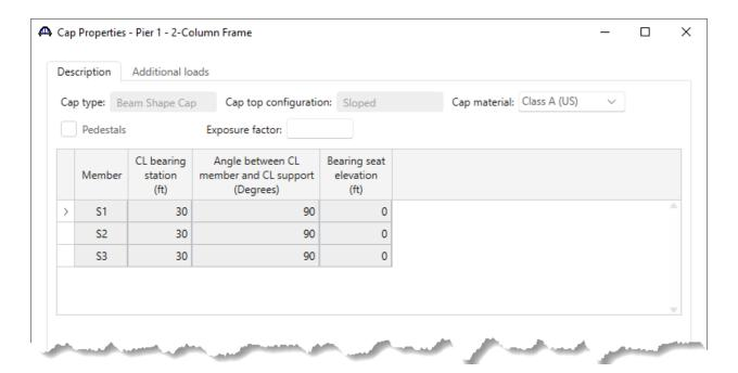
The **Additional loads** tab allows the user to define additional user defined loads on the cap. This example does not contain any additional loads on the cap. Click the **OK** button to apply the data and close the window.
