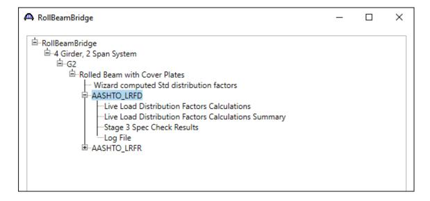
To view the LRFD spec check results, double click on the **Stage 3 Spec Check Results** under the AASHTO\_LRFD branch in this window. The following file opens.
