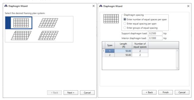
Click the **Finish** button to add the diaphragms. The **Diaphragm Wizard** will create diaphragms for all the girder bays in the structure. The diaphragms created for **Girder bay 1** are shown below.
