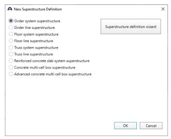
Select Girder system superstructure, click OK and the Girder System Superstructure Definition window will open. Enter the data as shown below.
