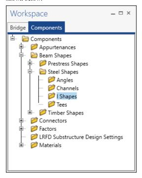
Click on the **I Shapes** node in the **Components** tree and select **New** from the **Manage** group of the **WORKSPACE** ribbon (or right mouse click on **I Shapes** and select **New** or double click on **I Shapes** in the **Components** tree). The window shown below will open.
