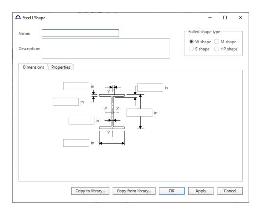
Select the **Rolled shape type** as **W shape** and click the **Copy from library...** button. The **Steel Shape Selection** window will appear. This window displays all of the steel shapes available in the library. The list can be sorted by clicking on any of the column headers (e.g. **Shape**, **Year**, **Depth** etc.). Select **W18x119** and click **OK**.
