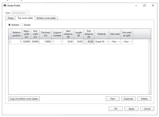
Click the **Copy to bottom cover plates** button to copy the top cover plate to bottom cover plate as shown below.
