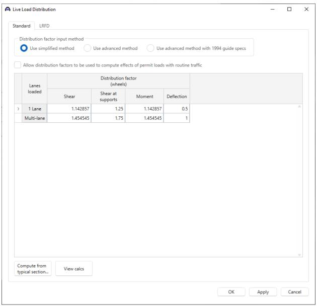
Live load distribution factor calculation details can be viewed by clicking **View Calcs** button. Click **OK** to apply the data and close the window.
