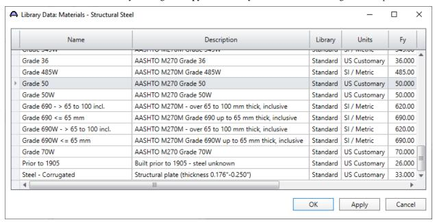
Select the **AASHTO M270 Grade 50** material and click **OK**. The selected material properties are copied to the Bridge Materials – Structural Steel window as shown below.
