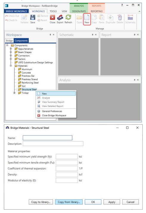
Add the structural steel material by clicking the Copy from library... button. The following window opens.
