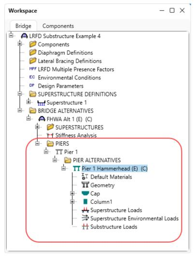
With the Pier alternative **Pier 1 Hammerhead** selected, click on the **Specification Check** button from the **Analysis** group of the **SUBSTRUCTURE DESIGN** ribbon to run a specification check analysis for this pier alternative as shown below.
