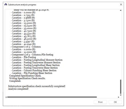
After the substructure specification check is completed, click on the **OK** button to close the window. Then click on the **Tabular Results** button from the **Results** group of the **SUBSTRUCTURE DESIGN** ribbon as shown below.
