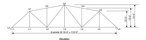
Modify the truss elevations and the second and fifth panels as shown below.
