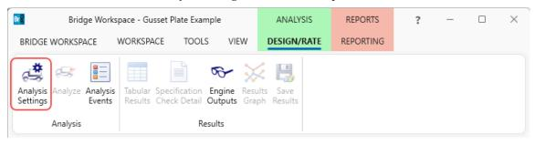
Click on the **Open template** button in the **Analysis Settings** window. The following window opens. Select the **LRFR Design Load Rating** template and click the **Open** button to apply the template.
