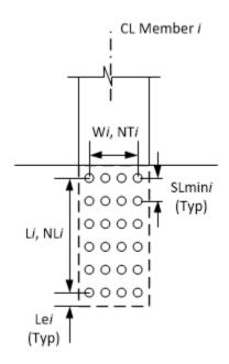
NL = Number of fasteners in a row along the longitudinal axis of the truss member.
