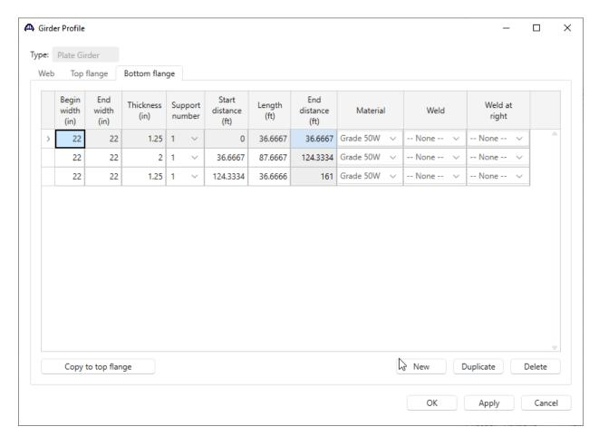
The last flange plate starts at a distance of 124.3334' and has a length of 36.6666'. This results in an end distance for this plate of 161.0000'. This member has a length of 161.0000' so the analysis should proceed successfully.
