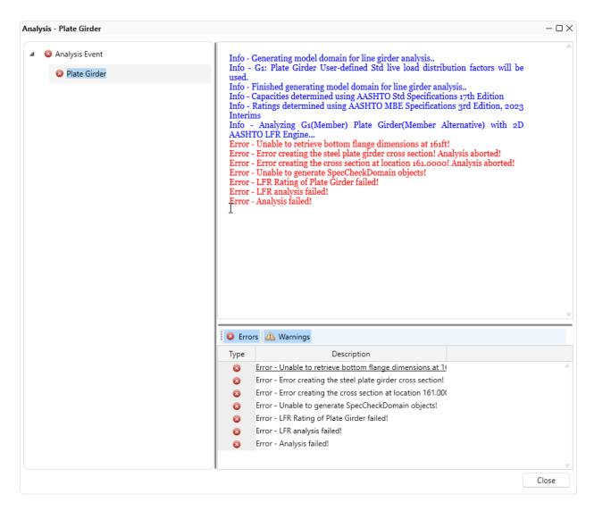
This error message tells us there was an error retrieving the flange plate properties to the left of the point at 161.00 ft. That is to be expected since we have a 0.006' gap at the end of the flange plate and our tolerance says that points must be within 0.001' of each other to be considered the same location.
