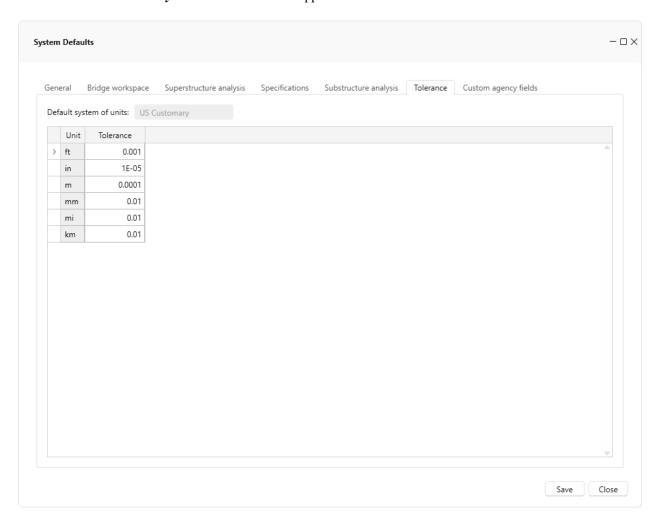
The tolerance for feet is shown as 0.001. That means that points that are within 0.001' of each other are considered to be the same location.
