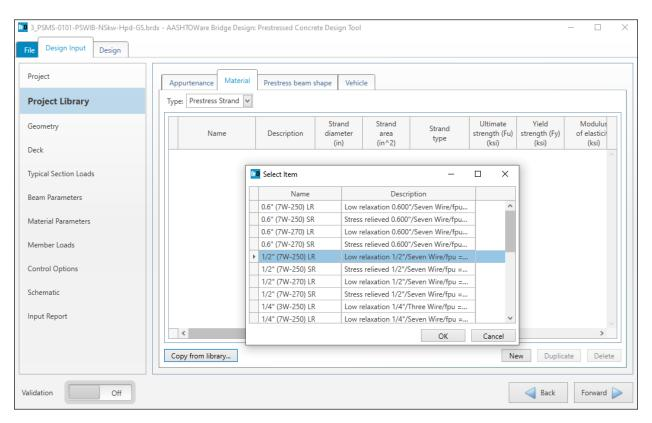
On the **Material** tab, select **Reinforcing Steel** for **Type** from the drop down menu and click the **Copy from library** button to copy the **Grade 60** reinforcing steel material definition from **File** | **Library** to the **Project Library**.
