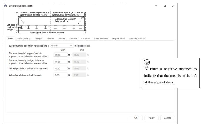
Enter the remaining structure typical section data as shown below.
