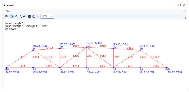
If floorbeams and stringers are described, BrDR will be able to compute the dead load of the floor system and apply it to the truss during the truss analysis.
